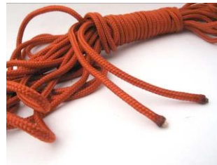
Melted 4mm Braided Nylon w/Core
