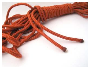
Melted 4mm Braided Nylon w/Core
